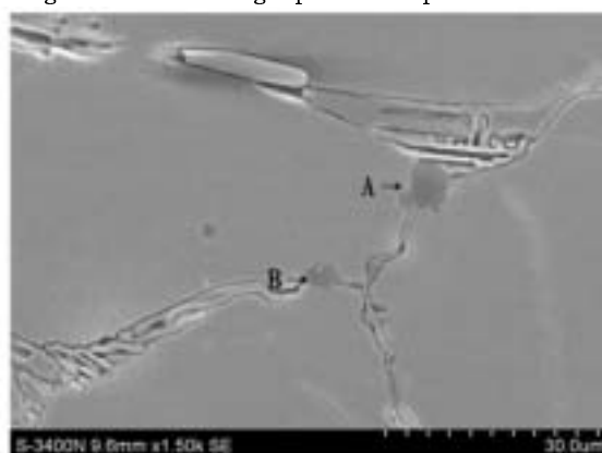
Fig. 11. SEM micrograph of sample Z3 and the micro-zone element analysis.
