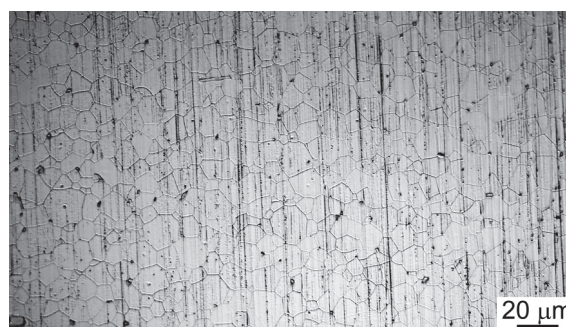
Fig. 7. Microstructure of Y_2O_3 ceramics obtained by slip casting and subsequent vacuum sintering at 1750°C for 10 hours
