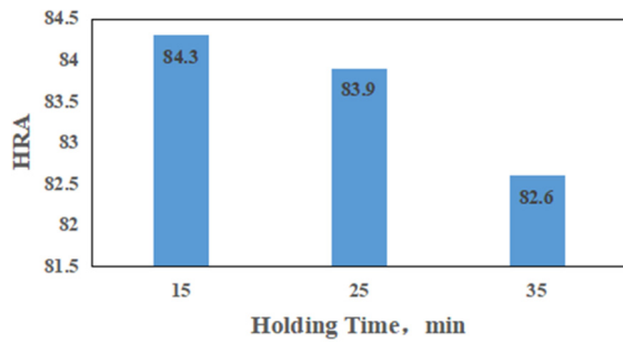
Fig. 4. Hardness of GCr15 steel specimens quenched at different holding time.
