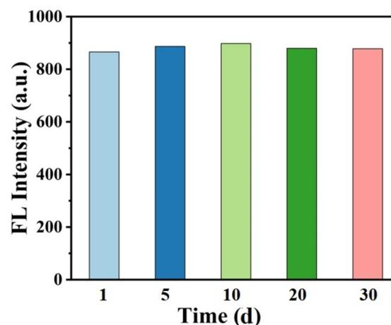
Fig.3. Stability of CuNCs@PVP placed at room temperature.
