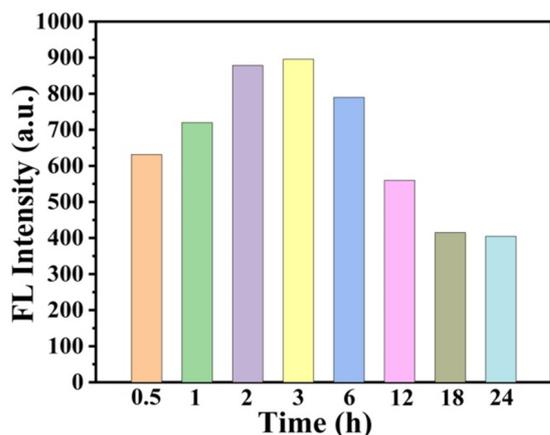
Fig. 1. Effect of reaction time on fluorescence intensity of CuNCs@PVP, the samples were synthesized at 200°C.
