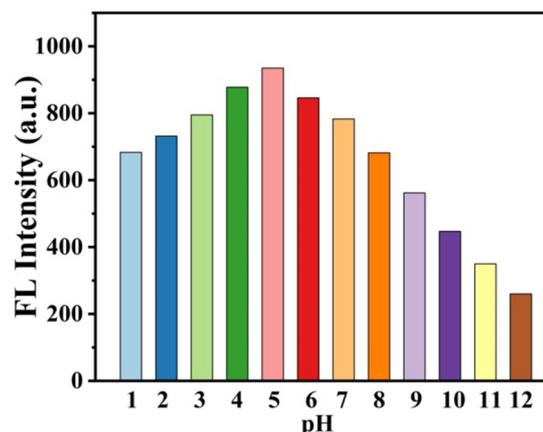
Fig. 2. Effect of reaction pH on fluorescence intensity of CuNCs@PVP, the samples were synthesized at 200°C and 2 h.
