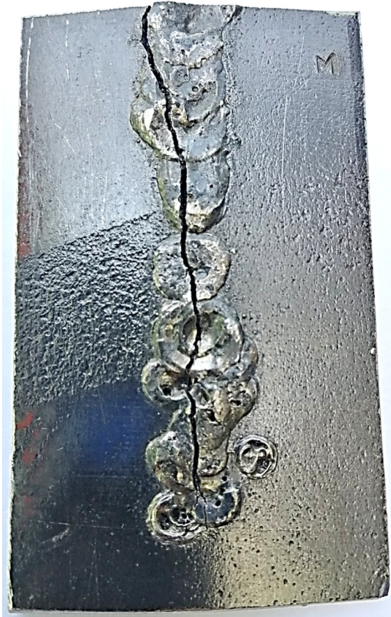
Fig. 4. The deposited layer of the composition 10% MS + 90% PG-10N-01 with a longitudinal crack
