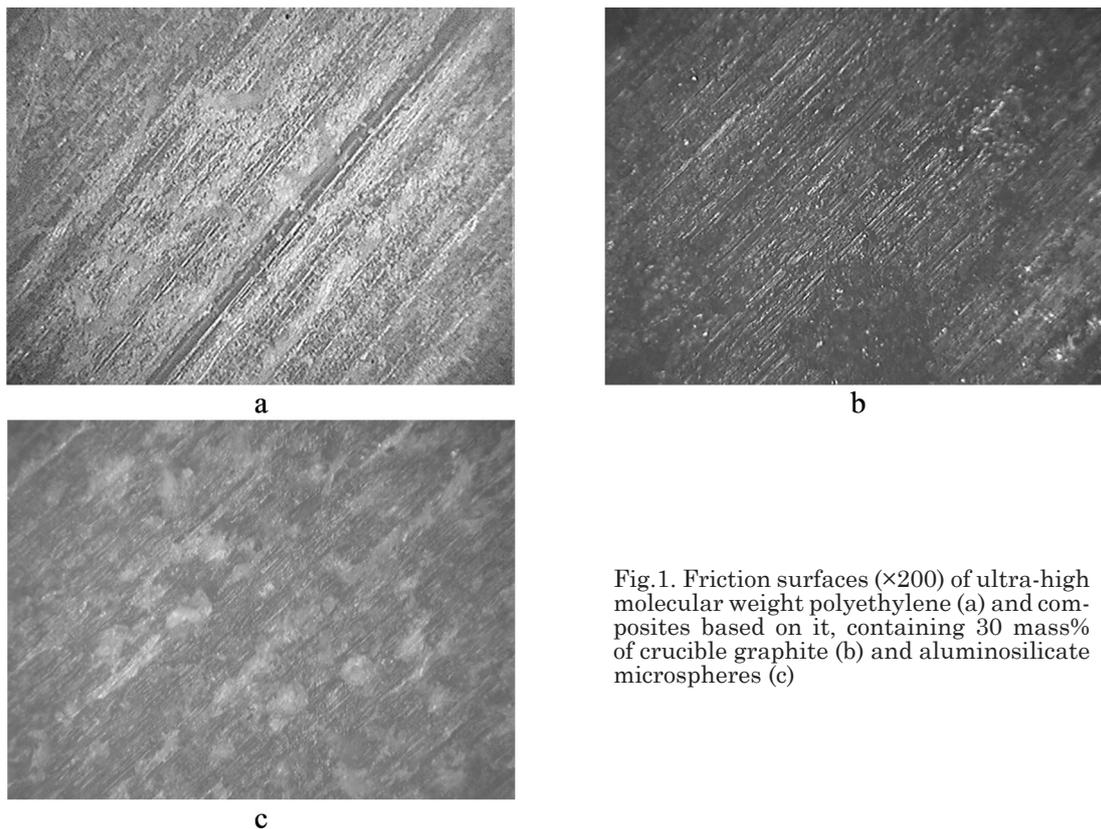
Fig.1. Friction surfaces ( $\times 200$ ) of ultra-high molecular weight polyethylene (a) and composites based on it, containing 30 mass% of crucible graphite (b) and aluminosilicate microspheres (c)
