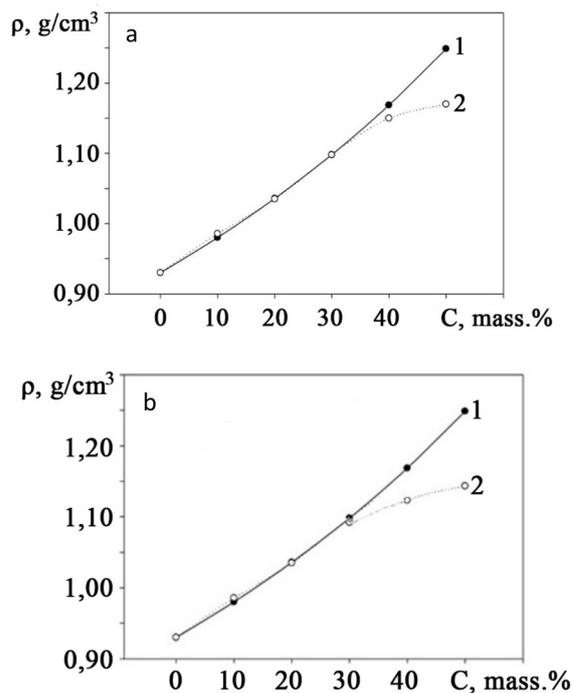
Fig. 3. Calculated (1) and experimental (2) density ( $\rho$ ,  $\text{g}/\text{cm}^3$ ) of ultra-high molecular weight polyethylene depending on the content ( $C$ , mass%) of crucible graphite (a) and aluminosilicate microspheres (b)
