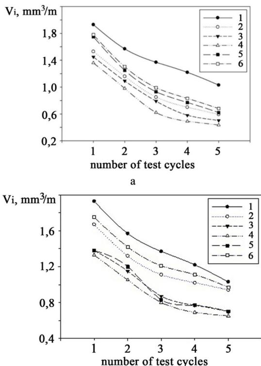
Fig. 2. Dependence of the index of abrasive wear ( $V_i$ ,  $\text{mm}^3/\text{m}$ ) on the number of test cycles for ultra-high molecular weight polyethylene (1) and composites based on it, containing 10 (2), 20 (3), 30 (4), 40 (5), 50 (6) of CG (a) and aluminosilicate microspheres (b)
