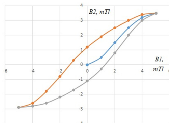
Fig.5. Hysteresis phenomenon in porous materials filled with iron oxides
